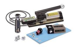
In this test, a dolly is glued to the epoxy and allowed to cure. The sample is then cored using a hole saw. A device with a piston is attached that pulls away from the substrate until it breaks.
